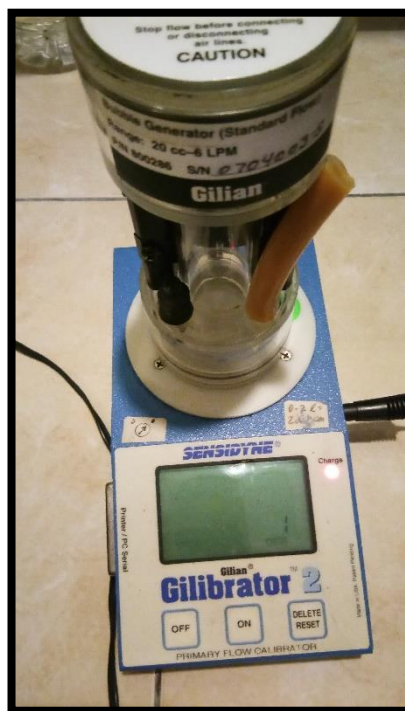
Figure 8: Gillian Sampling Pump Calibrator
